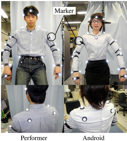
Fig. 6. The marker positions corresponding to each other
