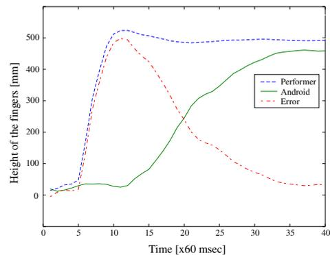
Fig. 10. The step response of the android
