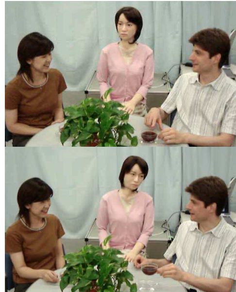
Fig. 1. Without understanding anything, the android robot Repliee Q1 (center) could give an impression of human presence by mimicking human autonomic and attentional movements. Repliee Q1 was a joint effort of Hiroshi Ishiguro's Intelligent Robotics Laboratory at Osaka University and Kokoro Co., Ltd.
