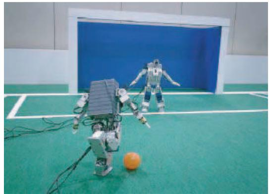
**Figure 8.** Fujitsu HOAP-1 robots are playing RoboCup soccer.
