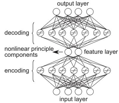
**Figure 4.** Target values presented at the output layer of a nonlinear principal component neural network are identical to input values. Nonlinear units comprise the encoding and decoding layers, while either linear or nonlinear units comprise the feature and output layers.
