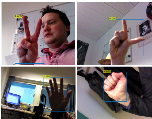
Fig. 13. Detection of hand gestures from the OUHANDS dataset in the presence of a human face (top left), background clutter (top right), illumination variation (bottom left), and change in hand orientation (bottom right).
